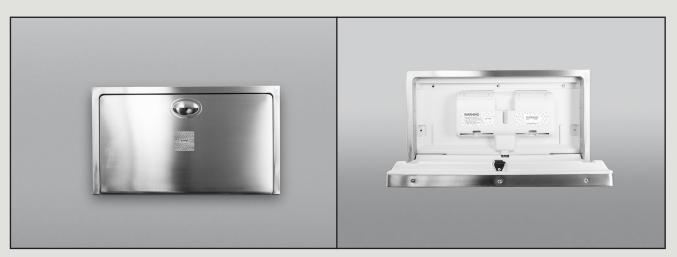
Colour Stainless Steel **Load Support** Up to 20kgs **Unit Weight** 23kg (net) Material 304 Stainless steel and polyethylene **Dimensions** 905W x 520H x 459D mm (open) 104D mm (closed which includes the internal wall recession) 10mm proud from wall when installed **Standards** Complys with EN12221 **Fixing** All fixings included + mounting template Warranty 12 Months
