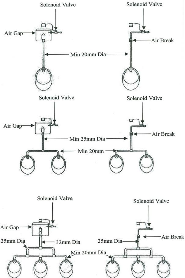
**Note;** Triple installations may require some form of water balancing to achieve uniform flushing to the three stalls.
