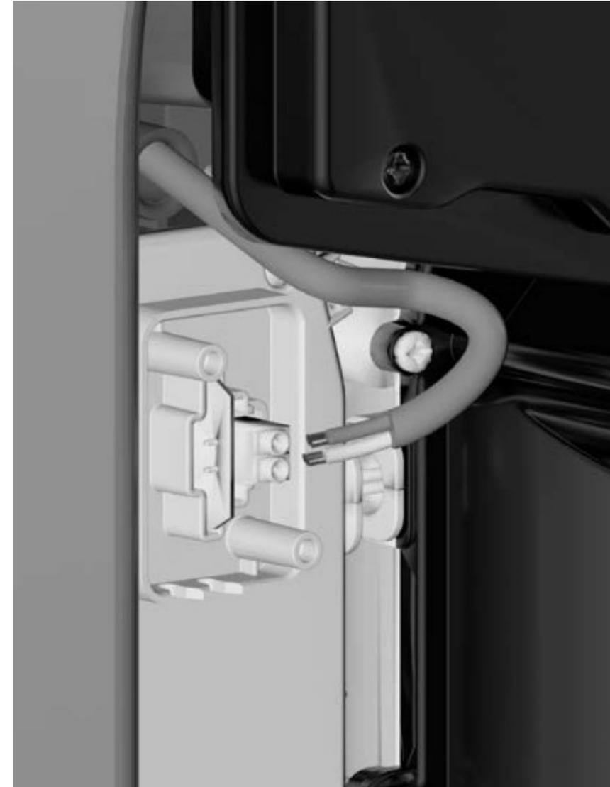
Once the cable has been passed through the hole, connect each end to its respective terminal, placing each one in the right path and then close the box.
