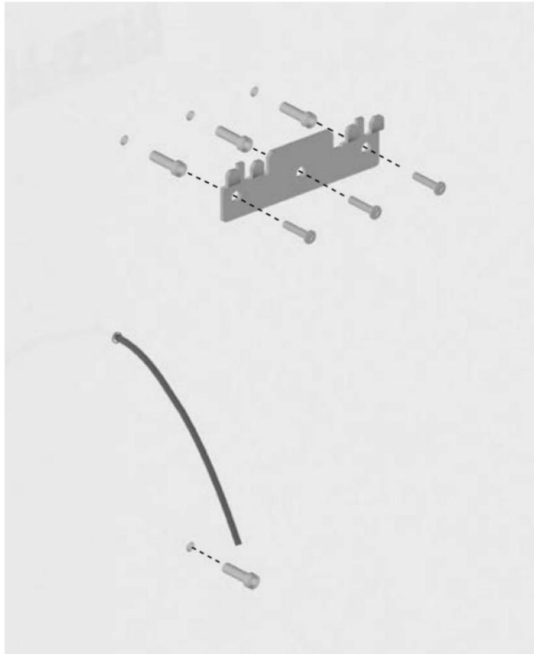
Once the marks have been made, attach the mounting bracket to the wall and prepare the cable to the electricity network.
