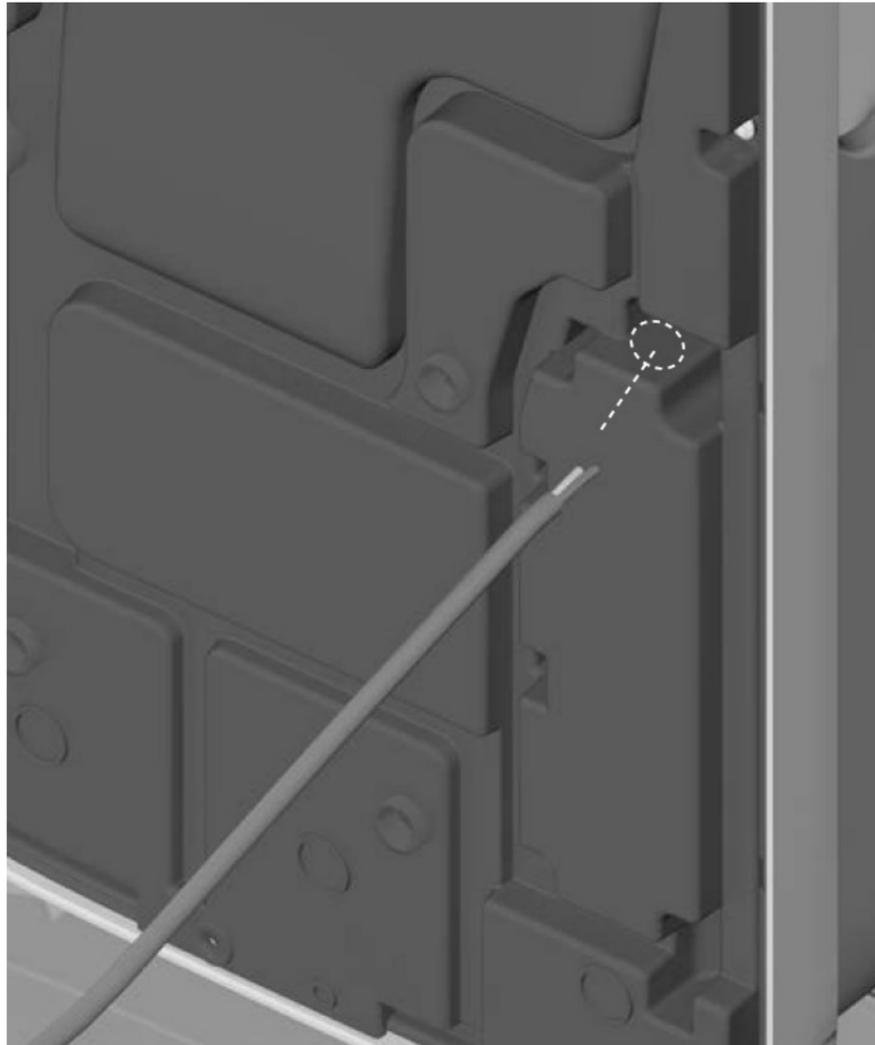
Introduce the electricity cable through the hole at the rear and pull it out from the front.
